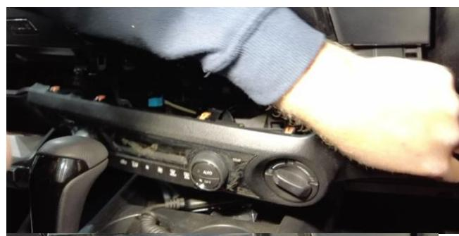
Route wiring from under glovebox area and into behind this central control panel switches area.
