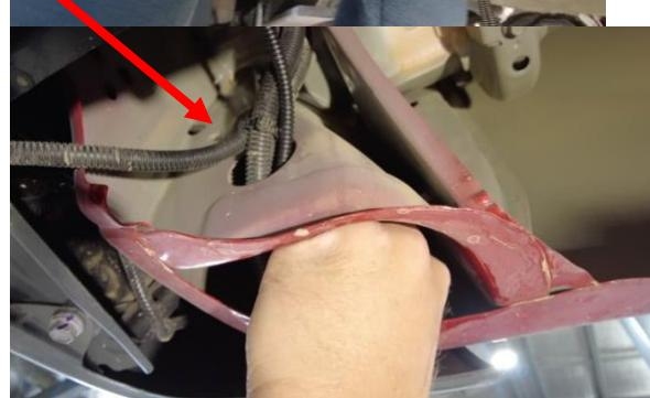
Find the fuse holder un-tape it, remove cover, remove fuse then plug in our 2 pin connector. Discard the lid and fuse. Push wire back up nice and neatly, cable tie if required.
