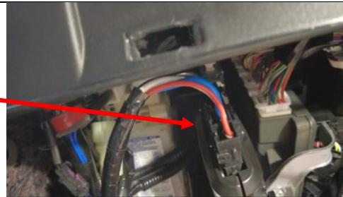
Direct the switch cable to the centre of the car.
