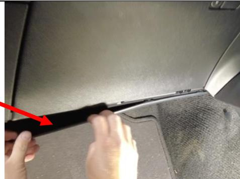
Find the Cable up underneath the glove box that you have fed through, and pull it through. The 'Y' split part of the loom should be at the grommet. As pictured.
