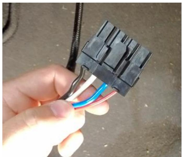
**Richards Auto – Electric Brake wiring harness to suit N80 HILUX & Redarc Tow Pro Elite V3**
